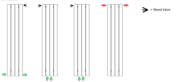
For Mid connection units, please cap off the four inlets ensuring a bleed valve is fitted to one of the upper two connections. For further information on installing your radiator valves, please consult the instructions provided with them.
