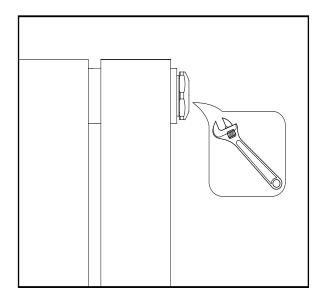
Please take care not to over tighten the bleed valve and blanking plug as this may damage the thread and/or the rubber O ring.
